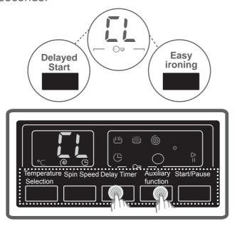
"CL" symbol will flash on the electronic display when activated. If any button is pressed while child lock is active, the "CL" symbol will blink on the electronic display.
