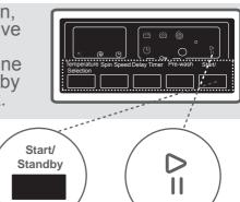
To avoid programme flow from being affected if programme buttons are pressed or programme button is turned when performing washing operation in your machine, child lock is available. Child lock will be activated in when both auxiliary functions 3 and 4 are pressed at the same time for more than 3 seconds.
