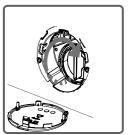
• While closing the pump cover, ensure that the parts on the inner side of the cover match the holes on the front panel side.
