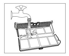
If necessary clean the filter with warm water using a brush. Close the filter.
