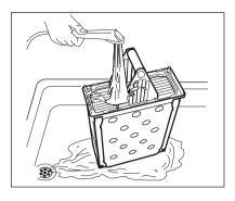
6. Clean the condenser in vertical position over a basin or paddling. Rinse through with a hand shower.
