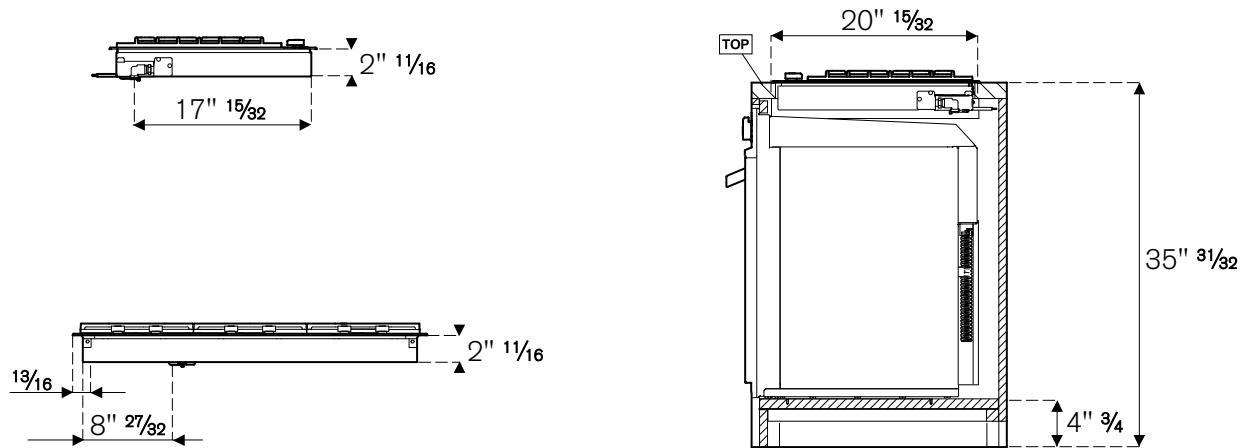
Bertazzoni recommends to operate the appliance after it has been installed in a cabinet. The kitchen cabinets shall be made of materials capable of withstanding temperatures at least 117°F (65°C) above room temperature in order to avoid possible damage to the cabinets during appliance usage. For further installation instructions refer to the installation manual.
