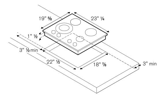
Bertazzoni recommends to operate the appliance after it has been installed in a cabinet. The kitchen cabinets shall be made of materials capable of withstanding temperatures at least 117°F (65°C) above room temperature in order to avoid possible damage to the cabinets during appliance usage. For further installation instructions refer to the installation manual.
