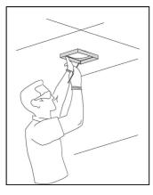
• Fix the upper horizontal support with 4 wood screws.
