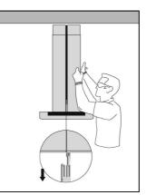
• The lower duct cover shall be secured to rangehood by 4 screws.
