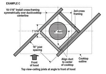
• Place the template in the ceiling considering the instructions for ceiling support structures.
