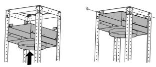
Measure from the bottom of the air deflector to the bottom of the hood outlet, as shown.
