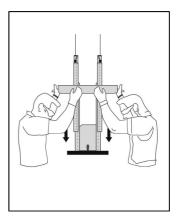
Place glass brackets using 2 screws by side.
