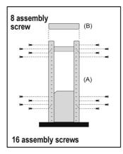
Attach a second vertical support set to adjust the vertical distance.
