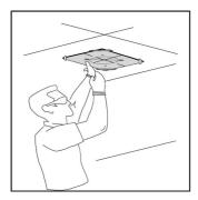
Mark with a pencil the hole locations for screws and duct in the ceiling.
