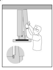
• Place lower duct covers using one plastic bracket at each vertex (4 needed).
