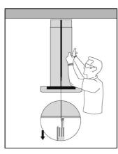
The lower duct cover shall be secured to rangehood by 4 screws.
