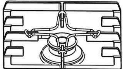
Examples of positioning of mini-trivet
