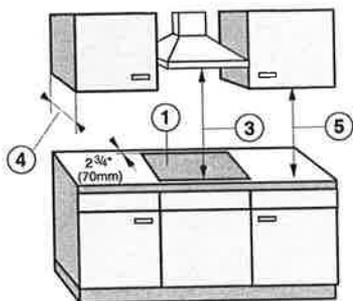
There must be a safety distance of at least 30" (760 mm), ③ between the appliance and any objects above it. The overhead cabinet depth, ④, if unprotected, must not exceed 13" (330 mm). The minimum distance of combustible surfaces located above and to the sides of the cooktop, ⑤, is 18" (457 mm).
