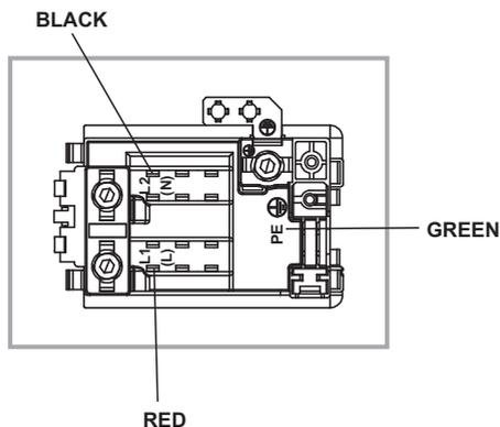
The power supply cable must be positioned away from direct heat sources. It should not be subjected to a temperature rise of more than 50°C above room temperature.
