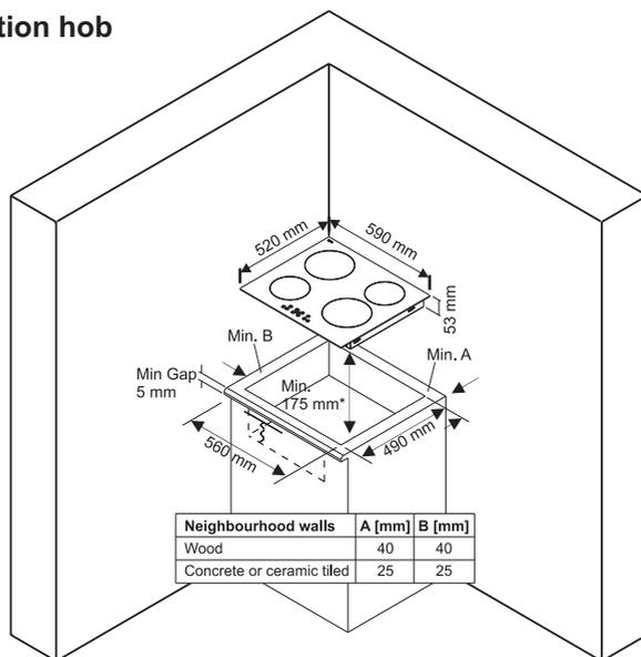
\* : In the case of installation over built in oven, distance should be min. 10 mm.
