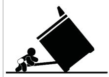
To reduce the risk of the appliance tipping, it must be secured and connected using the anti-tip device according to the installation instructions. Re-engage the anti-tip device if the range is moved.
