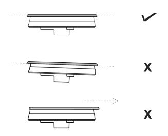
The burner grates must be properly placed inside the recess on the cooktop.
