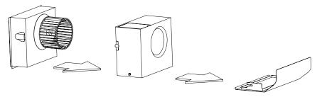
To remove the blower housing(s) and damper(s), first remove the E-Z Clean blower shield. The blower housing is removed for cleaning by unsnapping the suitcase latches (one on each side of the housing). Then, pull the housing forward and gently "tip" it downward to clear the blower wheel(s). The blower wheel(s) can be removed (if necessary) by using a 1/8" hex wrench. See part C of this section for details on how to clean the blower wheel(s).
