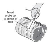
Figure 16: Probe in thickest area of food
