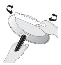
Figure 2: Checking pan for flat bottom
