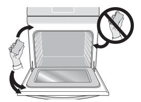
Figure 21: Clean around the oven door gasket
