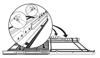
**6.** Extend and return the glide rack several times along the tracks to distribute the lubrication.
