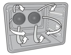
Figure 20: Air circulation in convection mode
