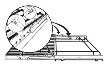
**4.** Extend and return the glide rack several times along the tracks to distribute the lubrication.
