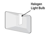
Figure 44: Wall oven Halogen light
