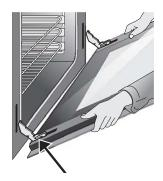
Figure 41: Holding door for removal
