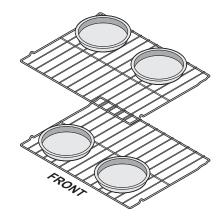
Figure 21: Pan spacing for convection baking
