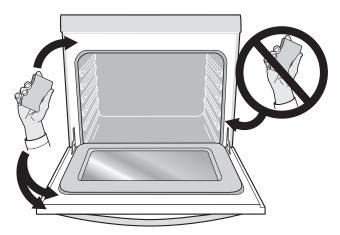
Figure 32: Oven door area to clean and not clean (gasket)
