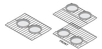
Figure 17: Single rack pan spacing (L), Double spacing (R
