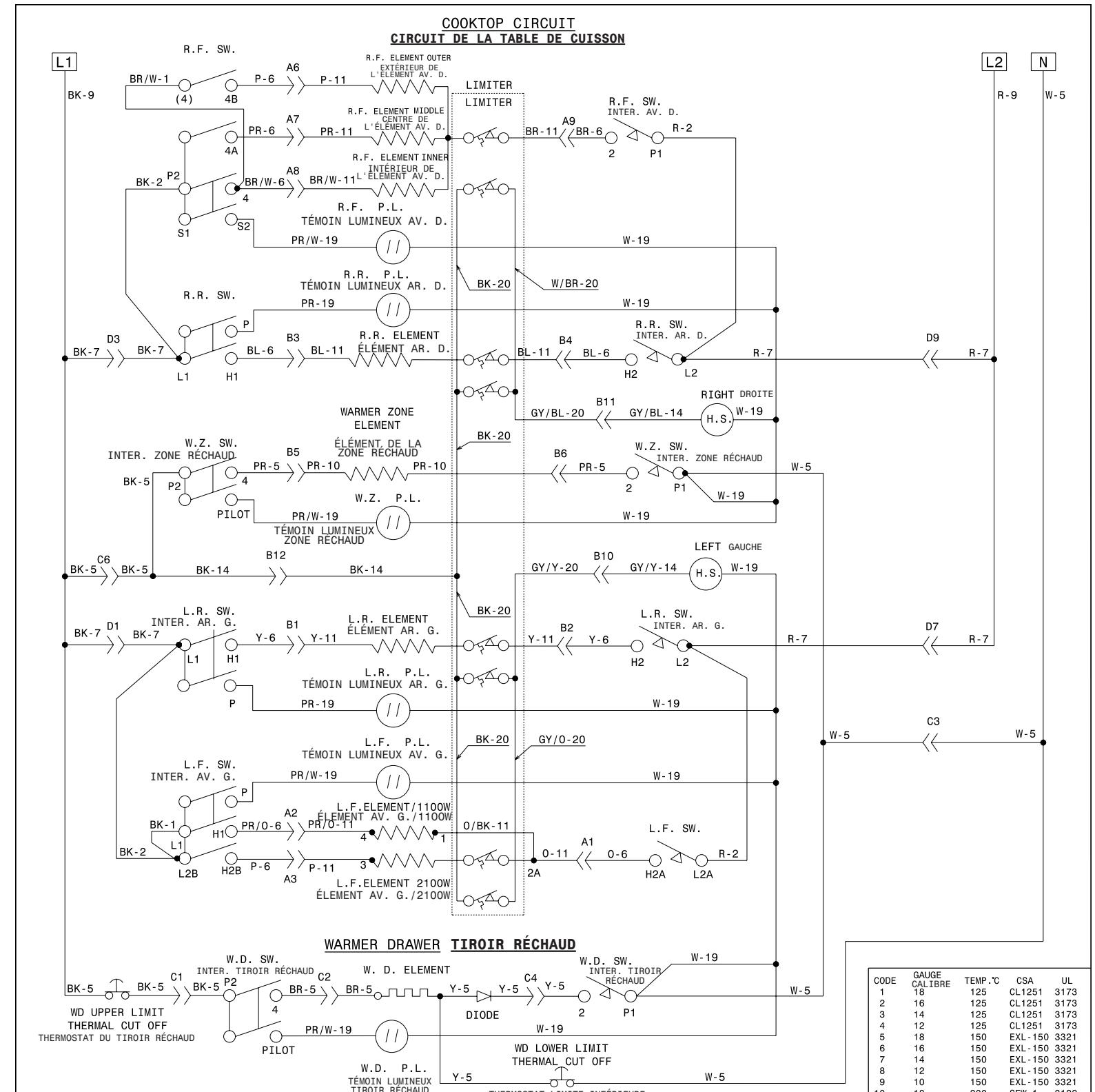
**NOTE:** WD UPPER LIMIT TCO & W.D. SWITCH REGULATE TEMPERATURE BASED ON SELECTION OF LOW/MEDIUM/HIGH.
