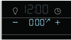
Figure 24: Probe inserted and ready to set temperature
