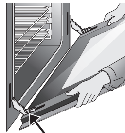
Figure 44: Holding door for removal
