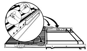
Extend and return the glide rack several times along the tracks to distribute the lubrication.
