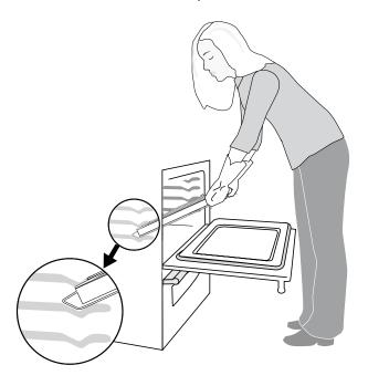
Figure 3 - Removing and replacing the oven glide rack.
