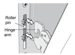
Figure 4 - Location of hinge arm and roller pin
