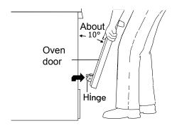
Figure 3 - Holding door for removal
