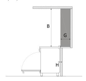
Shaded area behind range indicates minimum clearance to combustible surfaces, combustible materials cannot be located within this area.
