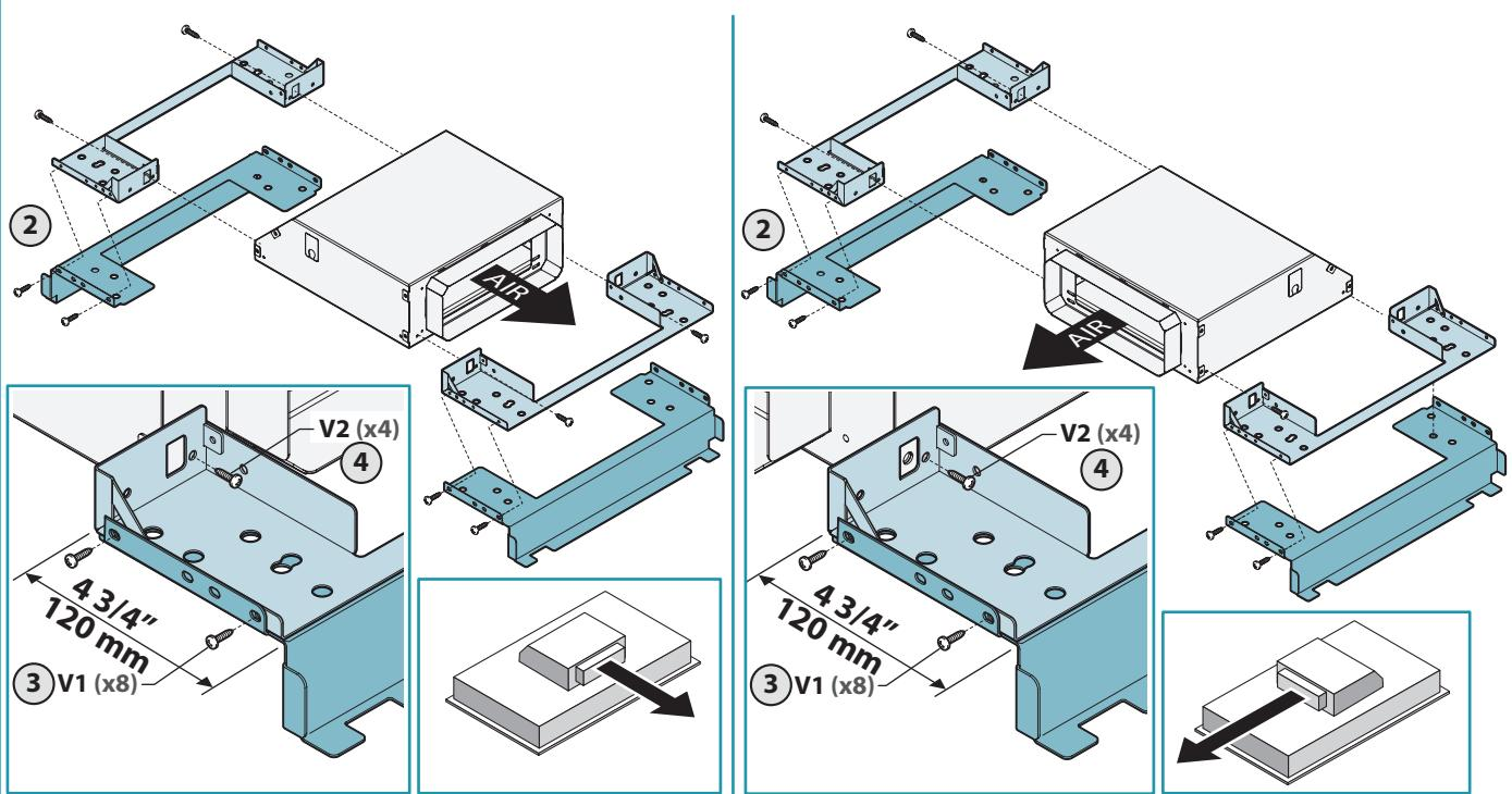
**EN** - Positioning the rectangular connection on the support frame (3).
