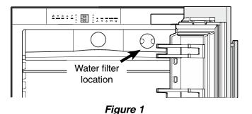
Replace the filter when the drop symbol appears on the temperature display.
