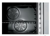
Two large-blade fans positioned on the diagonal axis and subsidiary air vents at the top and bottom of the oven cavity provide balanced airflow and even heat distribution.
