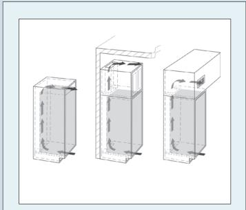
There must be an effective ventilation gap of at least 31 in² (200 cm²) per device at the air inlet and at the air outlet.
