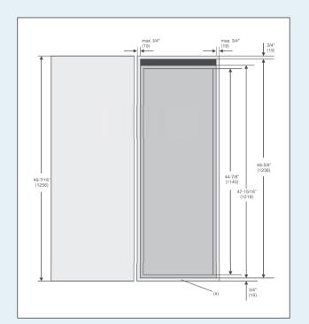
Total height of the cabinet (i.e. 49 7/16 in. (1256 mm)) plus thickness of the cover and floor plate (a) (normally 3/4 in. (19 mm)): 70 3/8 in.  $\pm$  3/4 in.  $\pm$  3/4 in.  $\pm$  47 15/16 in. (1218 mm  $\pm$  19 mm  $\pm$  19 mm  $\pm$  1256 mm)
