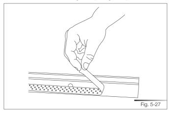
Fix the gasket to the dishwasher, inserting it in the seat on the sides towards the front (see fig. 5-28), and making sure that the long side of the gasket, the one with the hole for inserting the screw, is attached to the outside of the dishwasher; the hole in the long side must match the hole in the dishwasher (see ref. A fig. 5-29). Make sure the gasket adheres perfectly to the dishwasher.
