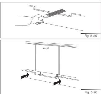
Before securing the dishwasher to the adjacent units, attach the gaskets to the sides.
