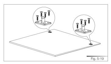
Drill holes for the panel handle using a drill with a suitable bit. Use the screwdriver to secure the door handle before hooking the panel to the dishwasher (see fig. 5-20).
