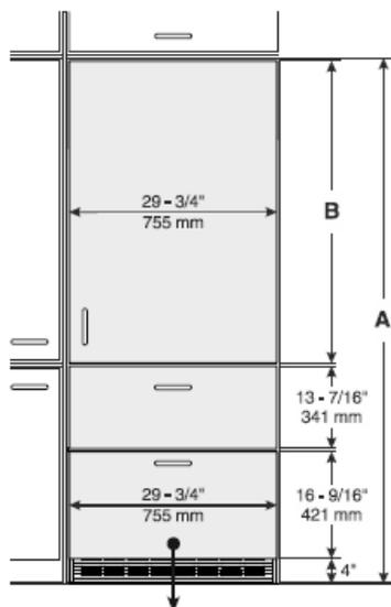
The height of this panel can be reduced by up to 2" to accommodate higher toe kicks
