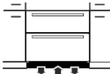
It is important to use the provided cover grille for the ventilation opening. This opening must not be covered with a cabinet base.
