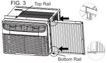
Your air conditioner is designed to install in standard double hung windows with opening widths of 24 to 36 inches (610 mm to 914 mm) (FIG. 4A, FIG. 4B).
