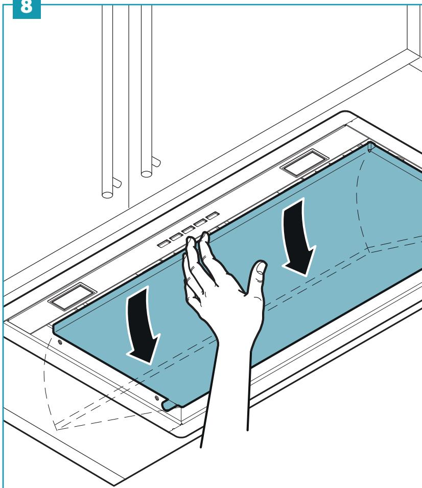
EN - Assembling standard active carbon filter: remove panel (8), remove metal filters (9), assemble active carbon filters (10).
