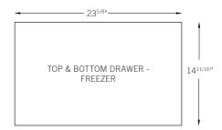
SPEC SAME PANEL FOR TOP & BOTTOM FREEZER DRAWERS. FOR BOTTOM DRAWER ROTATE PANEL 180°.
