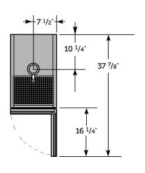
15" SINGLE TAP UNIT ACCOMMODATES (1) SLIM 1/4 BARREL OR (1) 1/6 BARREL.
