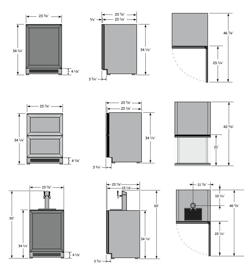
24" SINGLE TAP UNIT ACCOMMODATES (1) SHORT 1/4 BARREL, (1) SLIM 1/4 BARREL, OR (1) 1/6 BARREL. 24" DUAL TAP UNIT ACCOMMODATES (2) 1/6 BARRELS OR (1) SLIM 1/4 BARREL AND (1) 1/6 BARREL.
