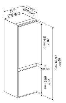
Installation before using the appliance Make sure there is enough space around the refrigerator to allow it work properly. A free space of 1cm (1/4inch) is required on the rear of the appliance so that the air can be circulated to cool the compressor and condenser. And 30cm (12inches) space above the refrigerator.
