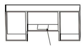
· Use the diagram above for correct placement of ductwork and electrical cut-out in cabinets.
