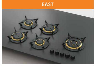
NUMBER OF BURNERS5POWER55,650 BTU/hMINIMUM CABINET WIDTH36 inchesMEASUREMENTS OF UNIT (L×W×H)20 × 33½ × 3½ inchesTOTAL HEIGHT3½ inchesMINIMUM COUNTER DEPTH24 inches
