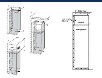
If the appliance is integrated in a fitted kitchen, the following ventilation requirements must be met: - The spacing fins on the back of the appliance are used to ensure sufficient ventilation. These must not lie in cavities or recesses in their final installation position. - Basically, the larger the ventilation gap, the more energy the appliance saves during operation. Do not restrict the air flow.
