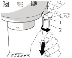
4. Remove the rubber nozzle (3) from the frother tube by pulling down on it.
