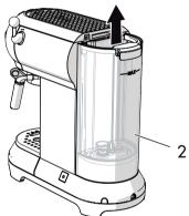
4. Fill the tank (2) with fresh, clean water directly from the faucet or by using a pitcher, being careful not to exceed the maximum level indicated on the tank.
