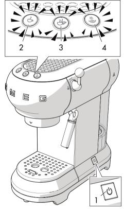
2. Lights (2) and (3) will flash to indicate that the machine is reaching the pre-set temperature. The espresso machine is ready for use as soon as the lights stop flashing.
