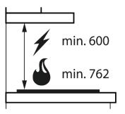
For optimal performance, the distance from the cooking surface to the bottom of the range hood should be between 24" and 30", unless otherwise noted. DO NOT install a range hood less than 24" above cooking surface.
