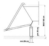
The free end should be positioned at a height of between 30 and 100 cm (11" 13/16 and 3' 3" 3/8), and should never be submerged in water.
